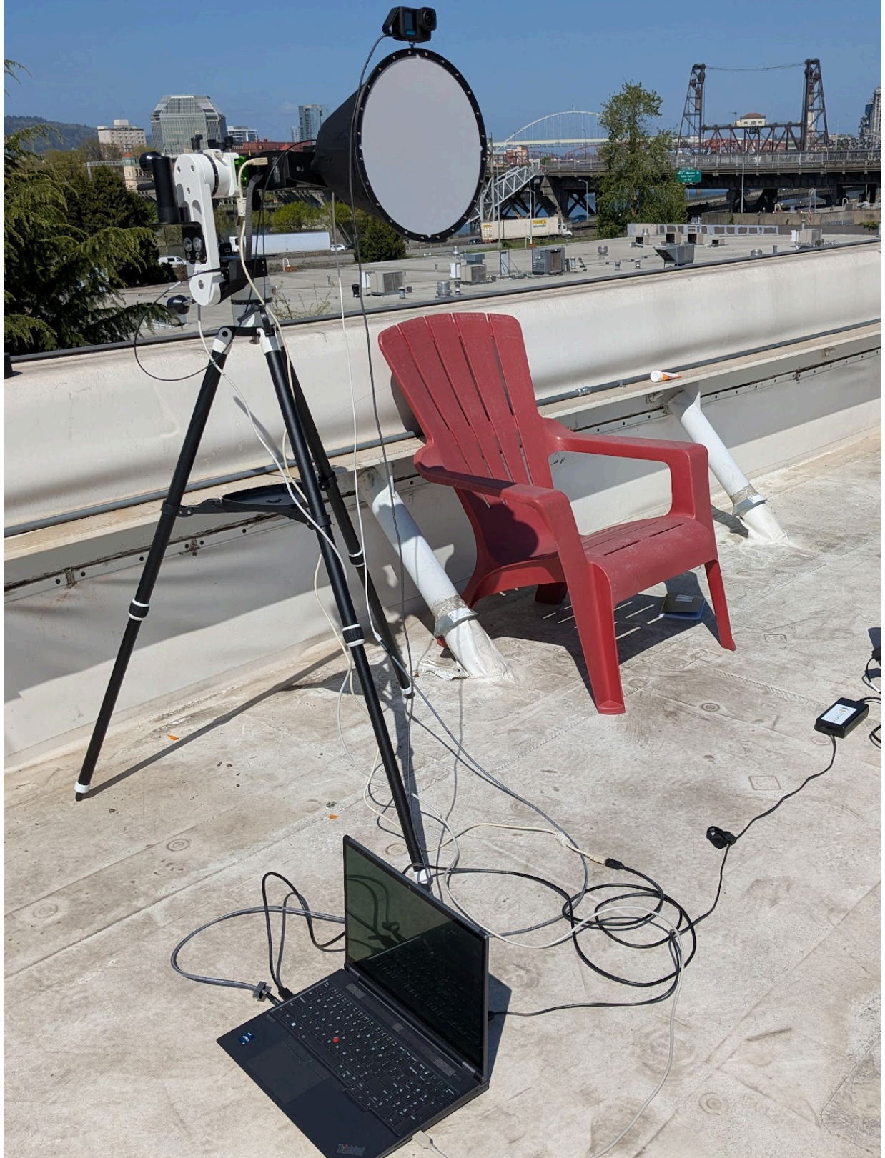
Figure 6: A hybrid test configuration combining controlled field-of-view restriction with uniform diffuse illumination.
